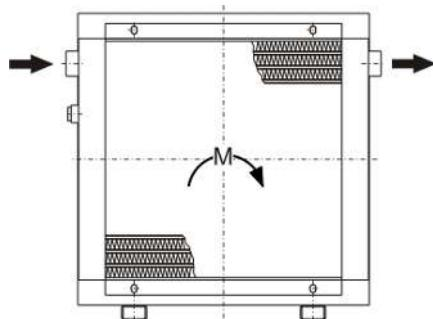
The oil inlet is on the left of the cooling battery. The oil outlet is always on the opposite side.
