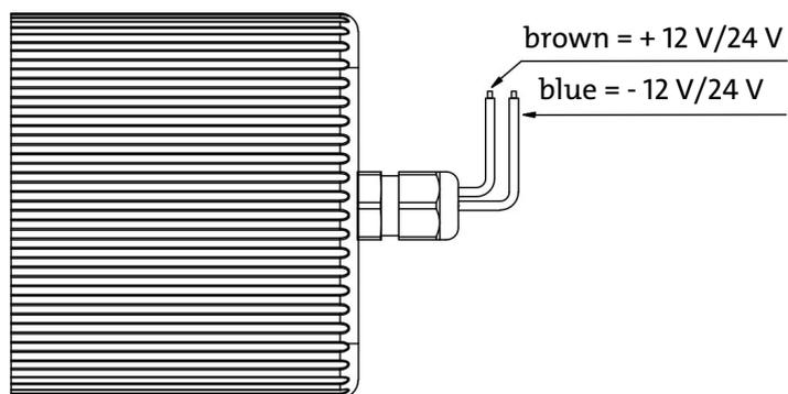
Fig. 2: Electrical connection P1.3 pumps
