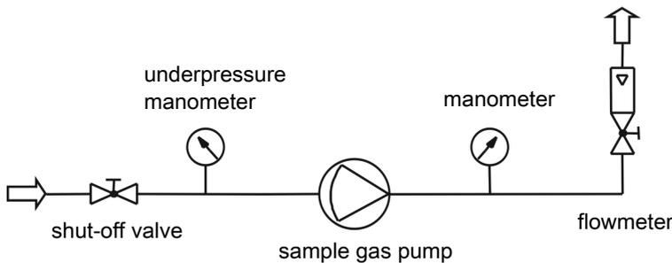
Fig. 1: Sample flow diagram of suitable monitoring
