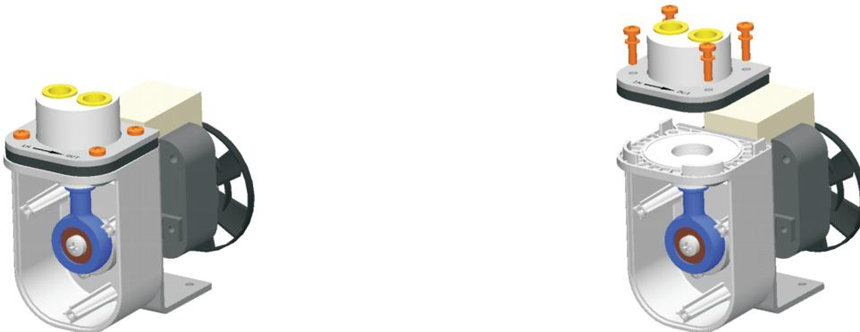
First detach the screw-in connections as described in chapter „Conversion to pump body pointing down“.
