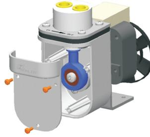
Loosen the 3 Torx screws (M3x8) on the front cover (Torx T10).
