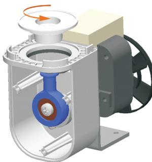
To replace the bellow carefully unscrew it from the connecting rod counter clockwise. Be sure not to lose any installed shims. Before reinstalling the bellow be sure it is not damaged. Reinstall hand tight in reverse order.
