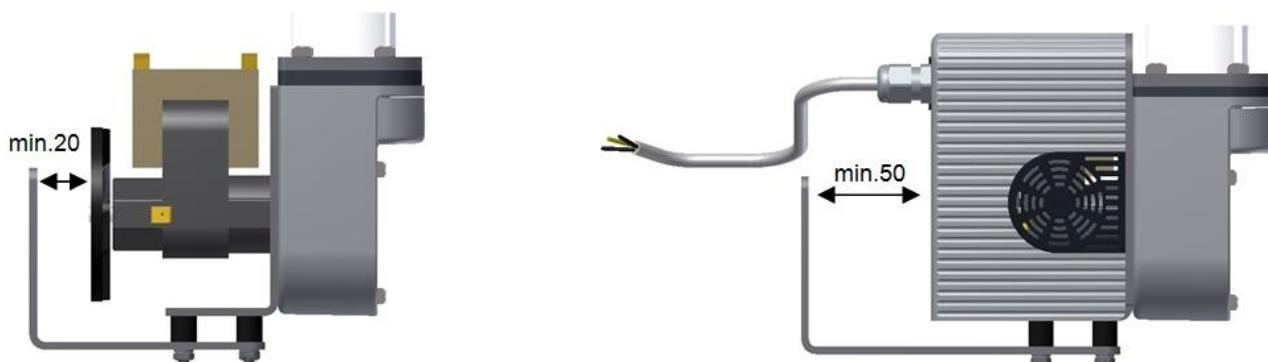
When installing the sample gas pump, always ensure an adequate amount of space between the motor and the back wall (20 mm).
