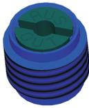
To assemble the sample gas pump, perform the steps in reverse order. When tightening the inlet and outlet valves be sure to observe the required tightening torque of max. 1 Nm. **CAUTION! Tightening the valves more will permanently deform the pump body, requiring replacement.**
