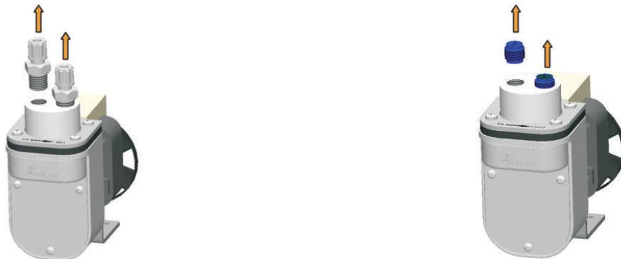
First detach the screw connections.
