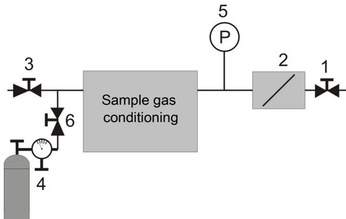
Fig. 7: Leak test set-up
