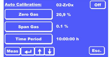
**On** - after applying the settings with **↵** the initial calibration will start and will then be repeated after the defined time period.
