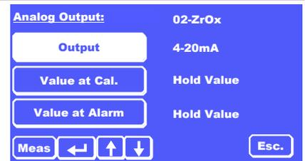
The analog output scaling varies according to the measuring range MR1 or MR2 settings. The lower value under MR1 is identical with that under MR2 and corresponds with the lower analog value. The upper analog value corresponds to the end value of the respective active measuring range. Please note, in automatic switchover the measuring ranges of the end value will automatically be adjusted. This must be considered when analysing the analog signal.
