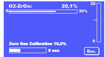
**Span Gas** Now select **Span Gas**, enter the concentration for the span gas and press **↵** to confirm.
