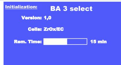
During initialisation you may touch the display to switch to measurement view, e.g. to configure the unit. The initialization progress is also displayed in measurement view: **WU 15 min** flashing
