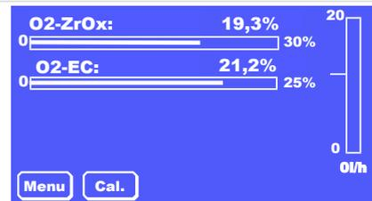
Wait at least **30 minutes** for the unit to warm up, then perform the first calibration. To measure very low concentrations it may be helpful to allow the unit to continue to warm up, **up to 2 h**.
