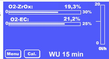
After initialization (**standard 30 min**) the measurement screen will appear.
