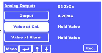
Note: With the setting for "Value at Alarm" taking priority over the setting "Value at Cal."; i.e.: If an error occurs during calibration, the measurement will be handled as configured in "Value at Alarm".
