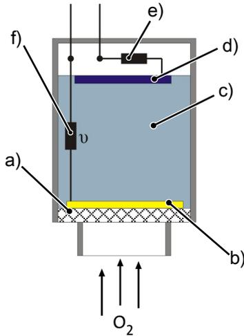
Fig. 3: Diagram of an EC cell
