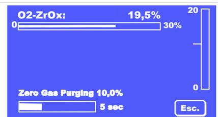
**Calibrate zero gas** This process will take the amount of time specified under **Cal.Period**. The process may be stopped at any time with **Esc.**
