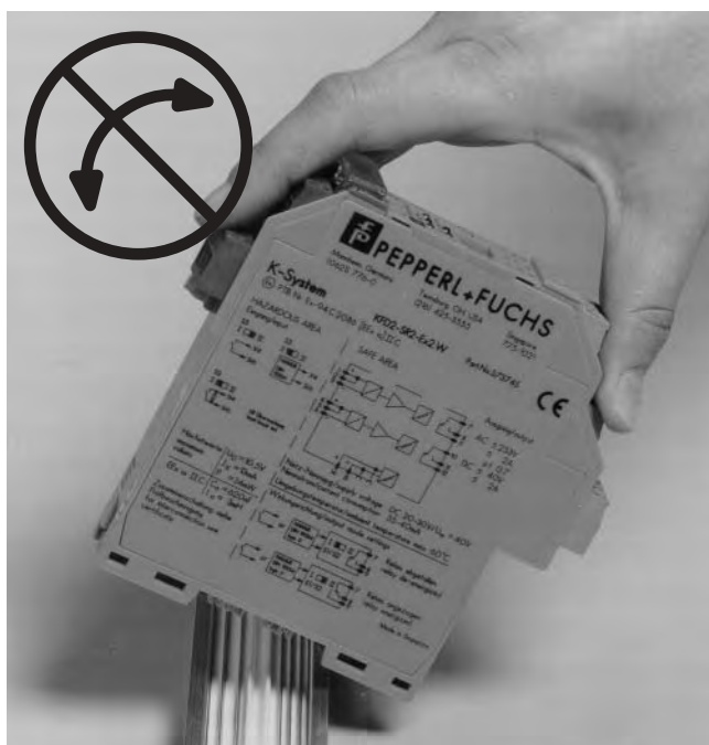
INCORRECT: Unit snapped on at an angle
