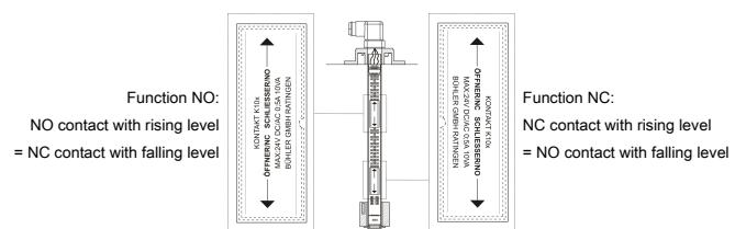
The contact logic assumes the level switch is installed in an empty tank, i.e. it is only in the operating position once filled.
