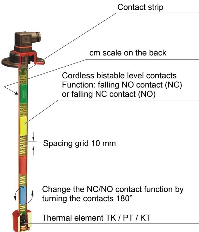
The contacts required for the float are mounted to a galvanically gold-plated with cm scale with plastic screws. The contact housings have different colours and may only be mounted to the contact strip in the following order.
