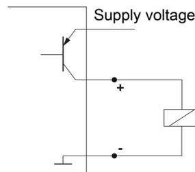
**Note:** When measuring the switching output with high-load measuring device inputs or when used as a frequency output, the load must be set to 10 kΩ between the output and earth (GND) to avoid faulty measurements.
