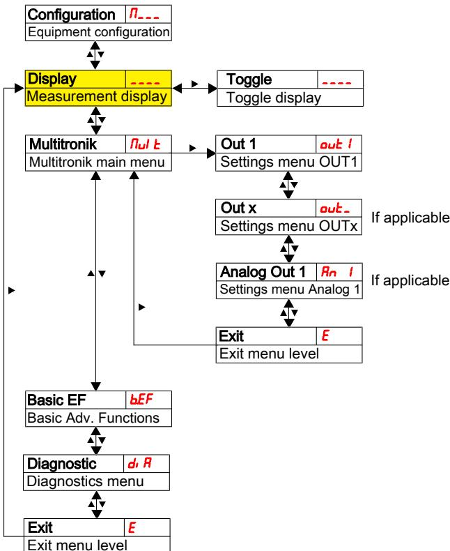
The individual menu items will not be shown if the option does not apply. Example: With a=0 the menu items for configuring the analogue output does not apply. You can then skip the description for this item.
