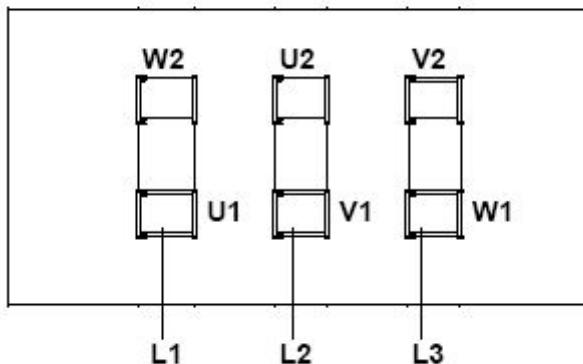
The direction of rotation can be changed by reversing any two phases.
