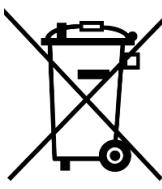
The crossed out wheelie bin symbol indicates the electric and electronic products bearing the symbol must be disposed of separate from household waste. They must be properly disposed of as waste electrical and electronic equipment.
