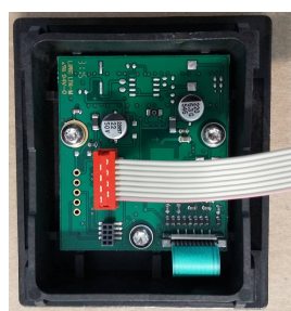
Installing the display, ribbon cable
