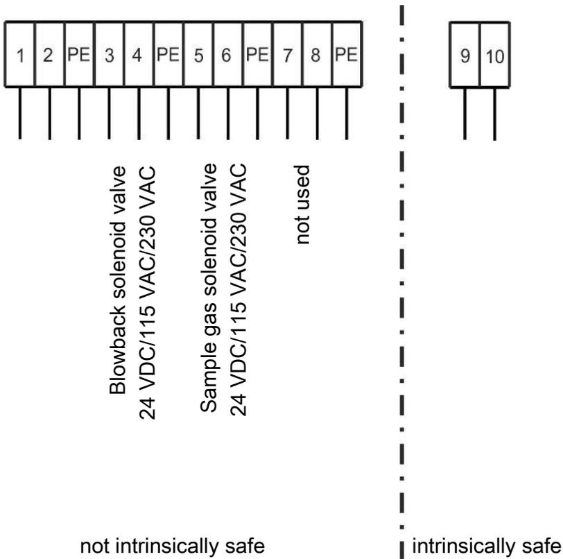
1.2 Terminal Diagram Terminal Box Limit Switch
