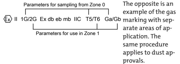
Please note, unlike the operating zone, the temperature class for sampling zone 0 is lower. This is also indicated by the ignition protection marking in the type plate.
