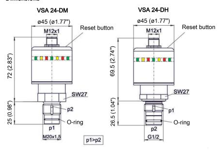
The reset button must be pressed after every filter change.
