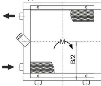
The oil inlet and outlet is always on the same side of the cooling battery. The connection on the opposite side must be closed.
