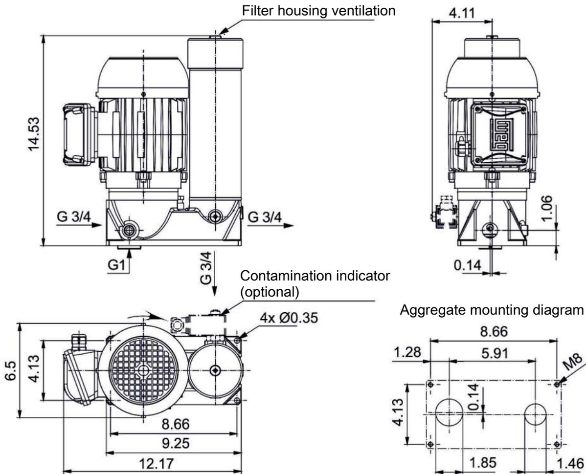
**Note:** When installing next to the oil reservoir please not the intake!
