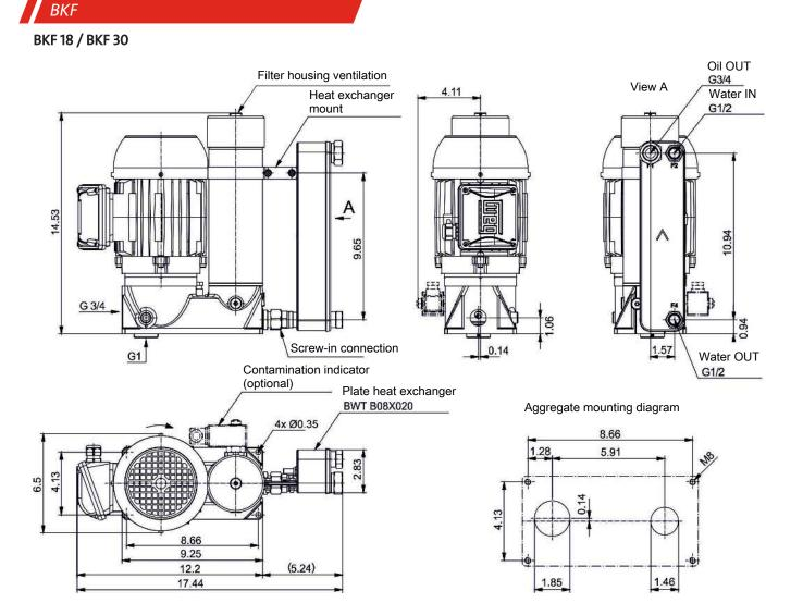
**Note:** When installing next to the oil reservoir please not the intake! When determining the bores on the reservoir be sure the contamination indicators remains visible!
