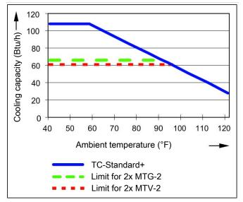
Note: The limit curves for the heat exchangers MTV-2 and MTG-2 apply to a dew point of 122 °F.
