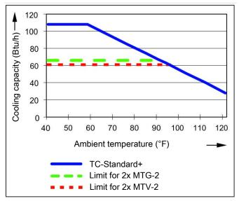
Note: The limit curves for the heat exchangers MTV-2 and MTG-2 apply to a dew point of 122 °F.
