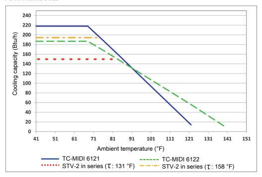
Note: The limit curves for the heat exchangers exchanger apply to a dew point of 122 °F.
