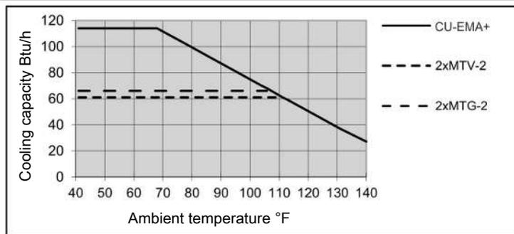
Remark: The limit curves for the heat exchangers MTV-2 and MTG-2 apply at a dew point of 122 °F. Depending on the installation version, the cooling capacity curve may vary.
