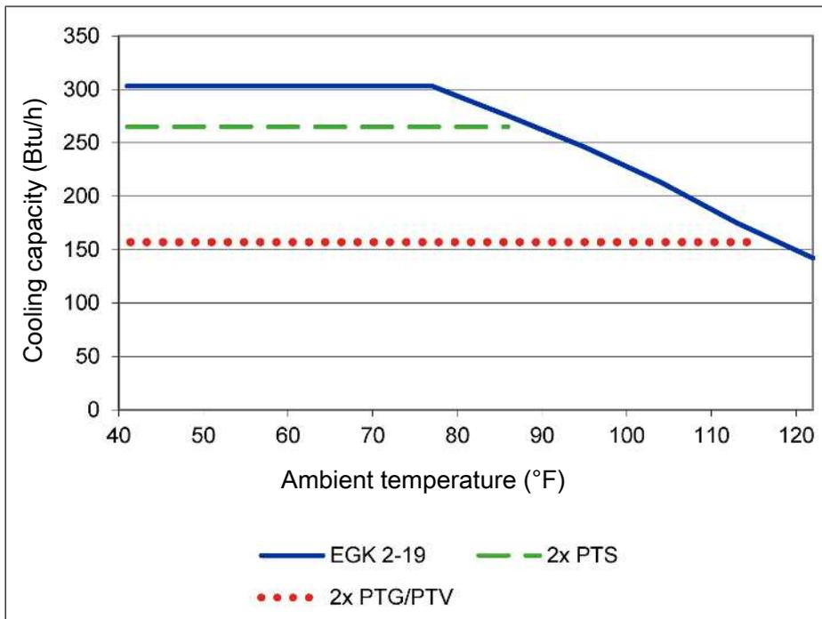
Note: The limit curves for the heat exchangers exchanger apply to a dew point of 104 °F.
