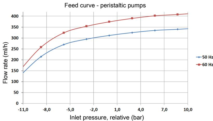
When operating the pumps with 60 Hz, the values increase by 20 %.
