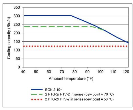
Remark: The limit curves for the heat exchanger apply to a dew point of 158 °F under standard conditions per DIN EN 15267-3:2008-03 and to a dew point of 122 °F under operating conditions.
