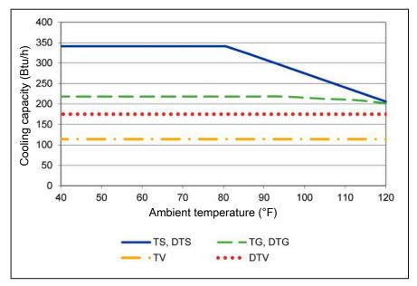
Note: The limit curves for the heat exchangers exchanger apply to a dew point of 149 °F.
