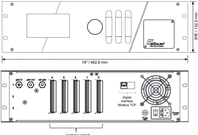
Analogue outputs (4 – 20 mA, Limit value + Status signals (Relay))
