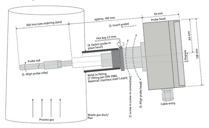
\* The fitting is welded to the waste gas flue and the Conversion nipple screwed in tightly. Then insert the BDA 02 all the way and secure in the desired position by socket screw.
