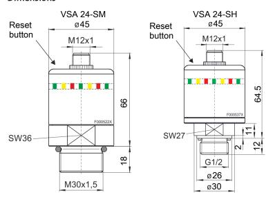
The reset button must be pressed after every filter change.
