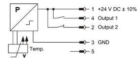
Output 1 = Alert at 2.2 bar (NO contact with rising pressure) Output 2 = shut-off at 2.9 bar (NC contact with rising pressure)
