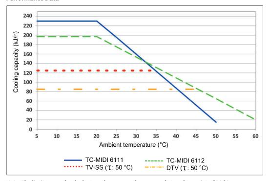
Note: The limit curves for the heat exchangers exchanger apply to a dew point of 50  $^{\circ}$ C.
