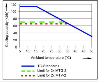
Note: The limit curves for the heat exchangers MTV-2 and MTG-2 apply to a dew point of 50 °C.
