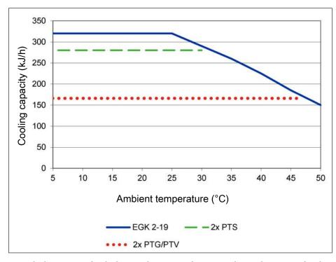
Note: The limit curves for the heat exchangers exchanger apply to a dew point of 40  $^{\circ}$ C.
