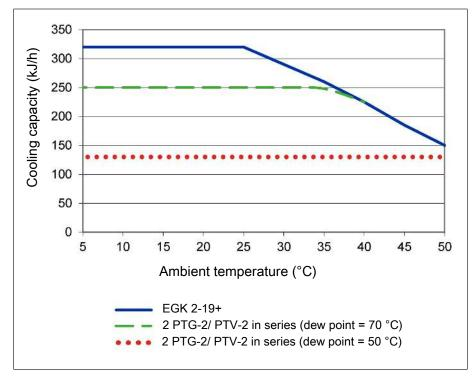
Remark: The limit curves for the heat exchanger apply to a dew point of 70 °C under standard conditions per DIN EN 15267-3:2008-03 and to a dew point of 50 °C under operating conditions.
