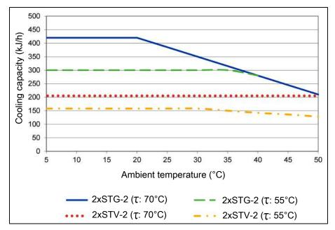
Note: The limit curves of the heat exchangers apply to different dew points ( $\tau$ ), see legend.
