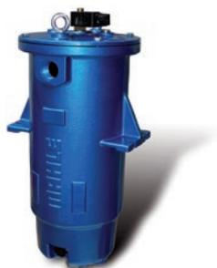
Our coalescer filter removes free water from hydraulic systems. It works without absorption media, simply and inexpensively. Specifically arranged special filter materials collect the small water droplets floating in the fluid and separate them out.
